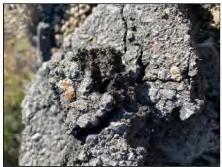
Figure 15: Asphalt fragments (tested for presence of coal tar) (2019)
