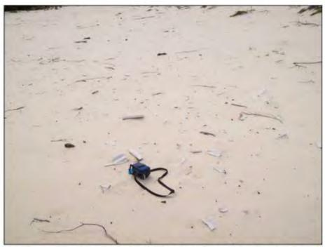
Figure 3: Fibro fragments (possible asbestos containing material (ACM)) observed in the eastern portion of Lot 11 (2009)
